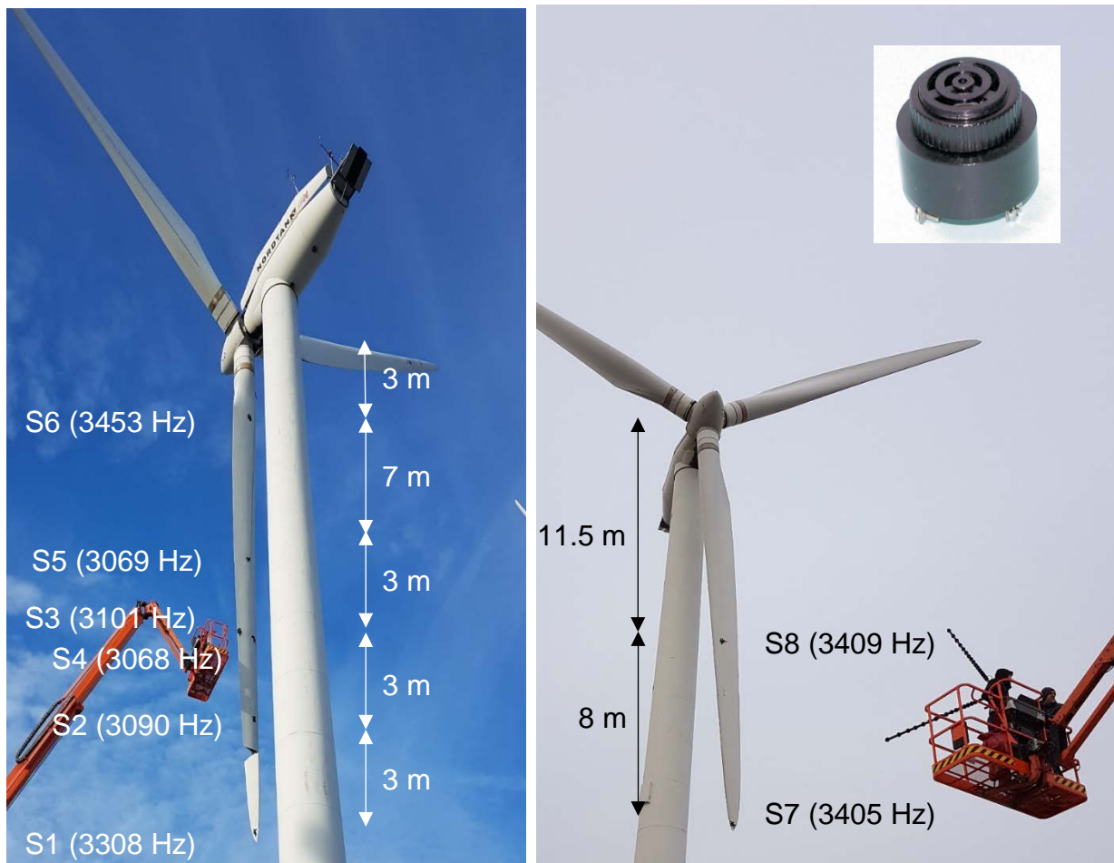
Figure 2. The location and tone frequency of the 8 speakers. Inset: one of the speakers.
