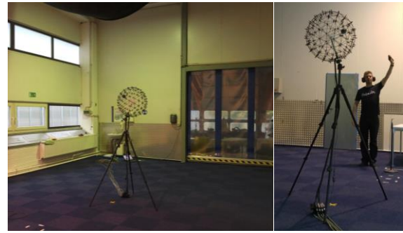
Fig. 11: RIR measurement at ADAM Audio
