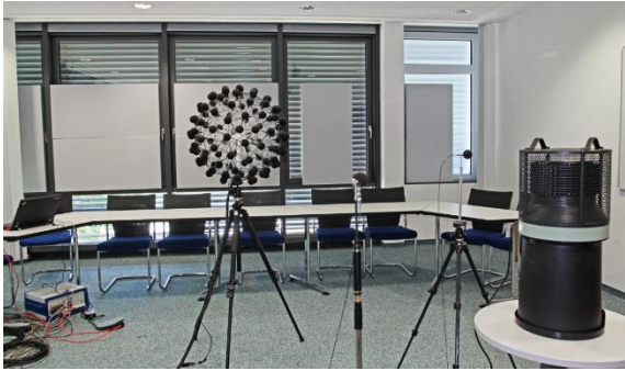
Fig. 20: Measurements setup in meeting room with constant power source and spherical microphone array
