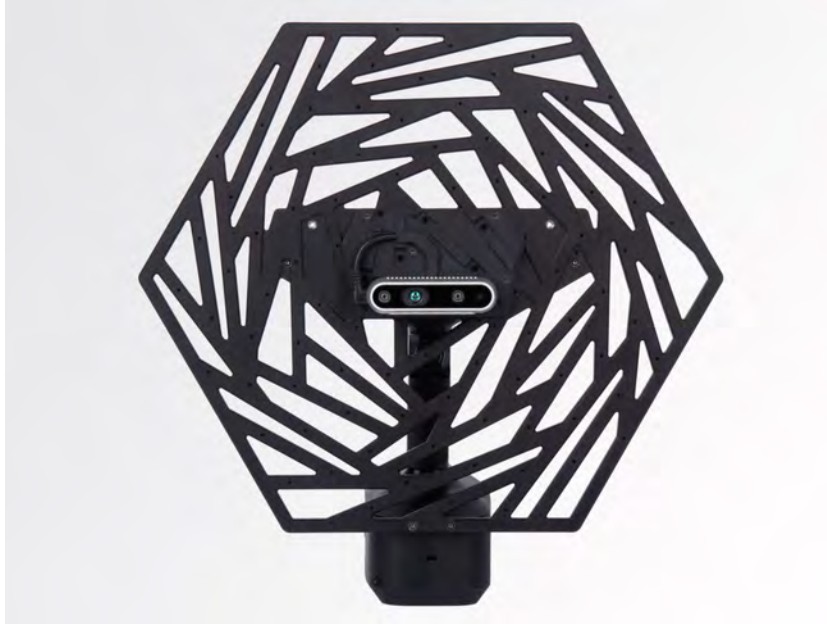
Figure 1: Mikado , a hand-held acoustic camera which consists of 96 MEMS microphones arranged in two sunflower spirals
