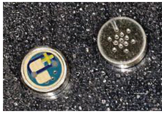
Figure 2 – typical electret microphone capsule
