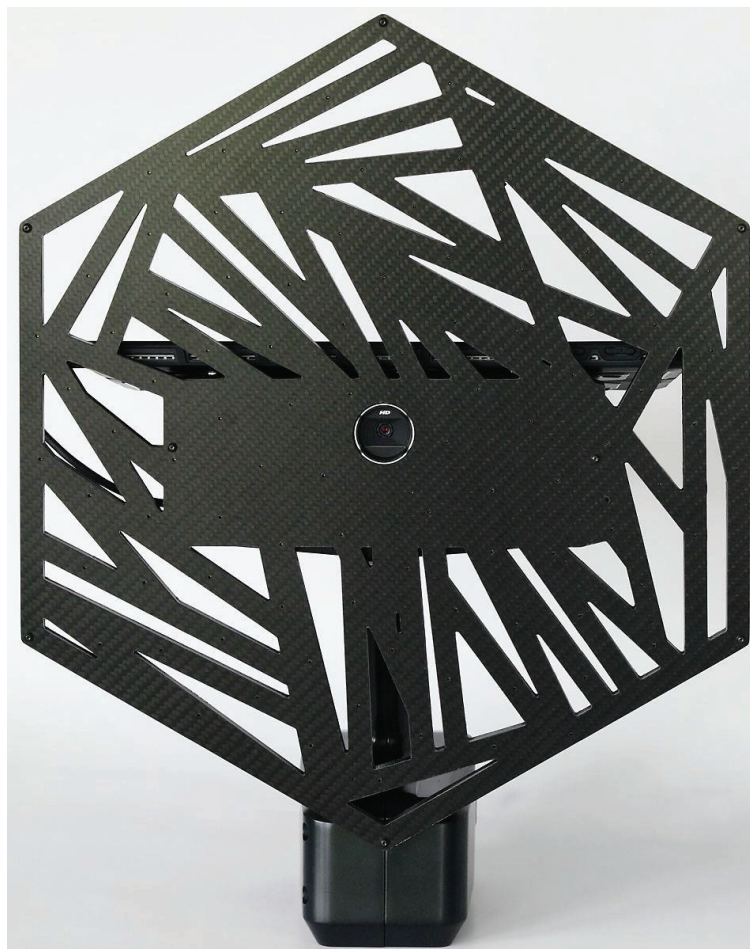
Figure 17 – Acoustic Camera with 96 digital MEMS microphones
