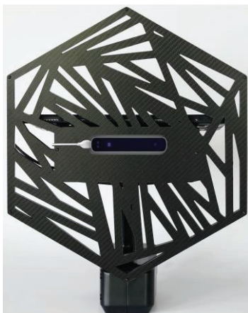
Figure 9 – Acoustic Camera Mikado with 96 digital MEMS microphones with Structure Sensor 3D scanner.
